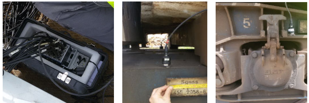
Figure 7. Dynamic tests of Sgnss wagon: DAQ and accelerometers on the platform and bogies.
