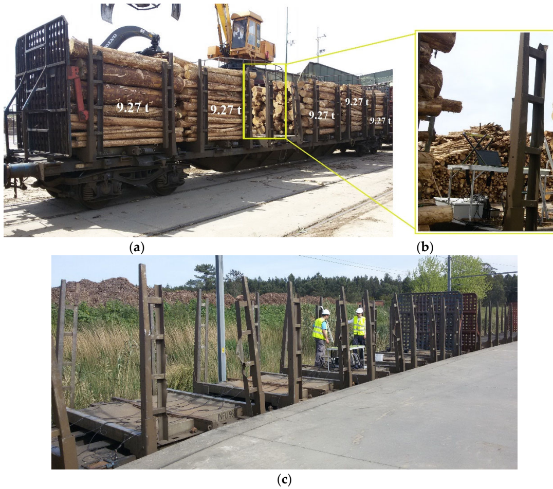
Figure 5. Dynamic tests of Sgnss wagon: (a) loaded configuration, (b) detail of the central stowage, (c) unloaded configuration.
