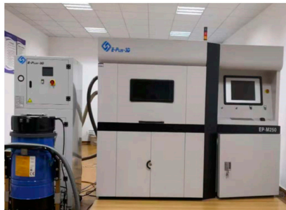
Figure 3. SLM forming principle and forming equipment EP-M250.
