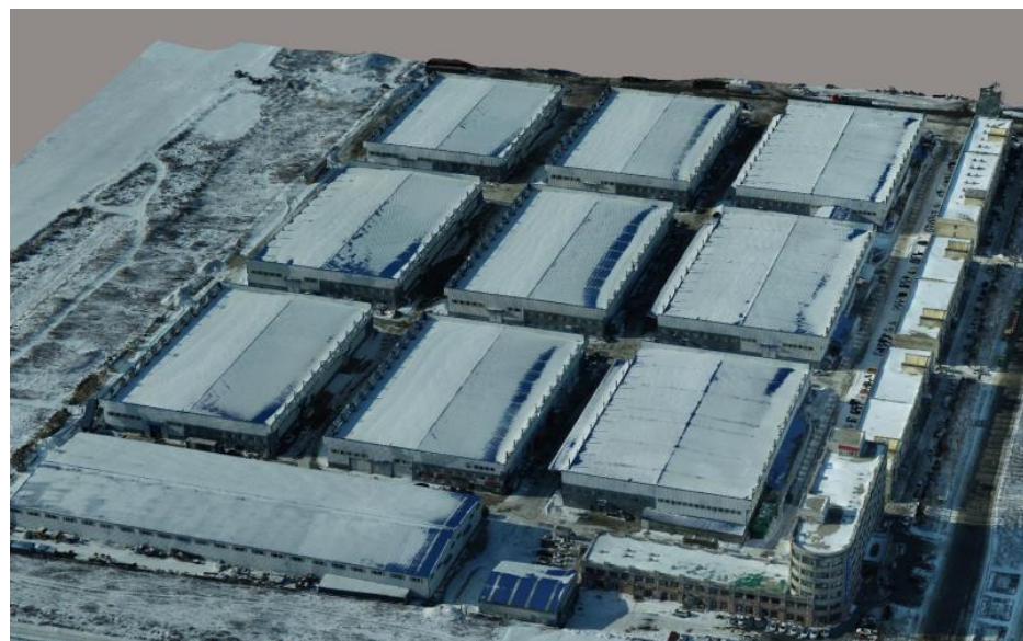
Figure 1. Three-dimensional model of snow distributions on a group of buildings in Harbin, China.
