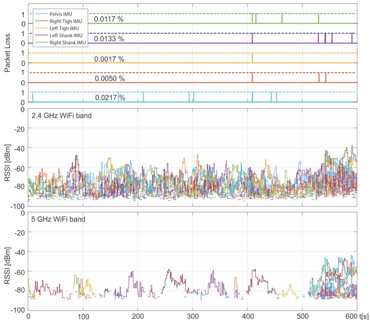
Figure 7. Top plot shows the measured packet loss for the IMU units attached to the pelvis, right/left thigh, and right/left lower leg. The middle plot shows the RSSI signal levels for various 2.4-GHz Wi-Fi band channels. Bottom diagram shows the RSSI signal levels for various 5-GHz Wi-Fi band channels.
