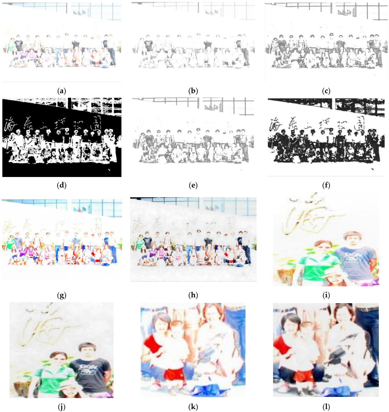
Figure 3. (a) Original image; (b) original radiance map I^h(i) ; (c) map of the mean radiance \mu_i ; (d) map of the standard deviation \sigma_i ; (e) the guidance map generated by (6); (f) the visualized guidance map c_i ; (g) the result obtained using the guidance map shown in (e); (h) the result obtained using the guidance map shown in (f); (i–l) the comparison of the details of figures (g,h), respectively.
