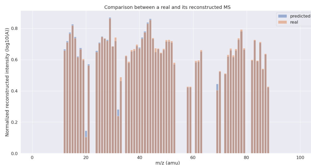
Figure 2. Comparison between a normalized reconstructed spectrum using the GA and the real one.
