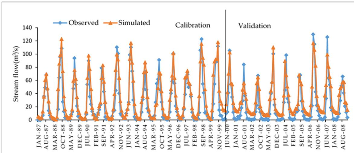
Figure 6. Monthly simulated and observed streamflow for calibration and validation using GLUE.
