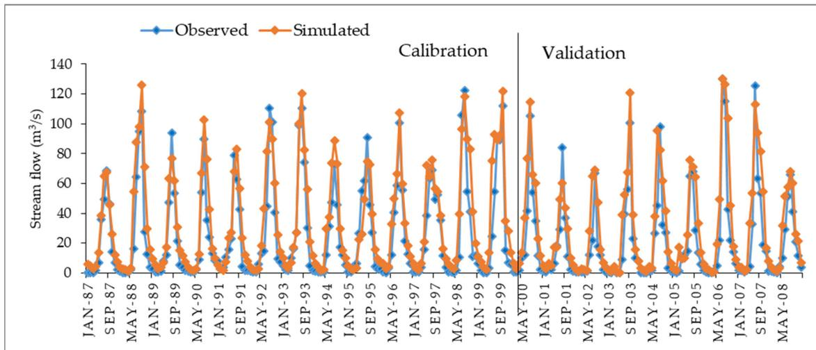
Figure 5. Monthly simulated and observed streamflow for calibration and validation using SUFI-2.
