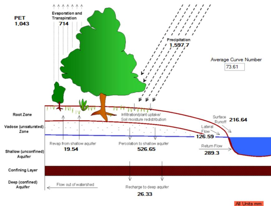
Figure 11. Pictorial representation of Soil and Water Assessment Tool (SWAT) output.
