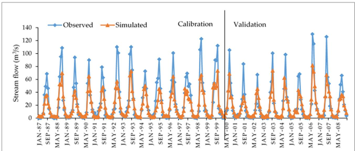
Figure 8. Monthly observed and simulated stream flow using PSO.
