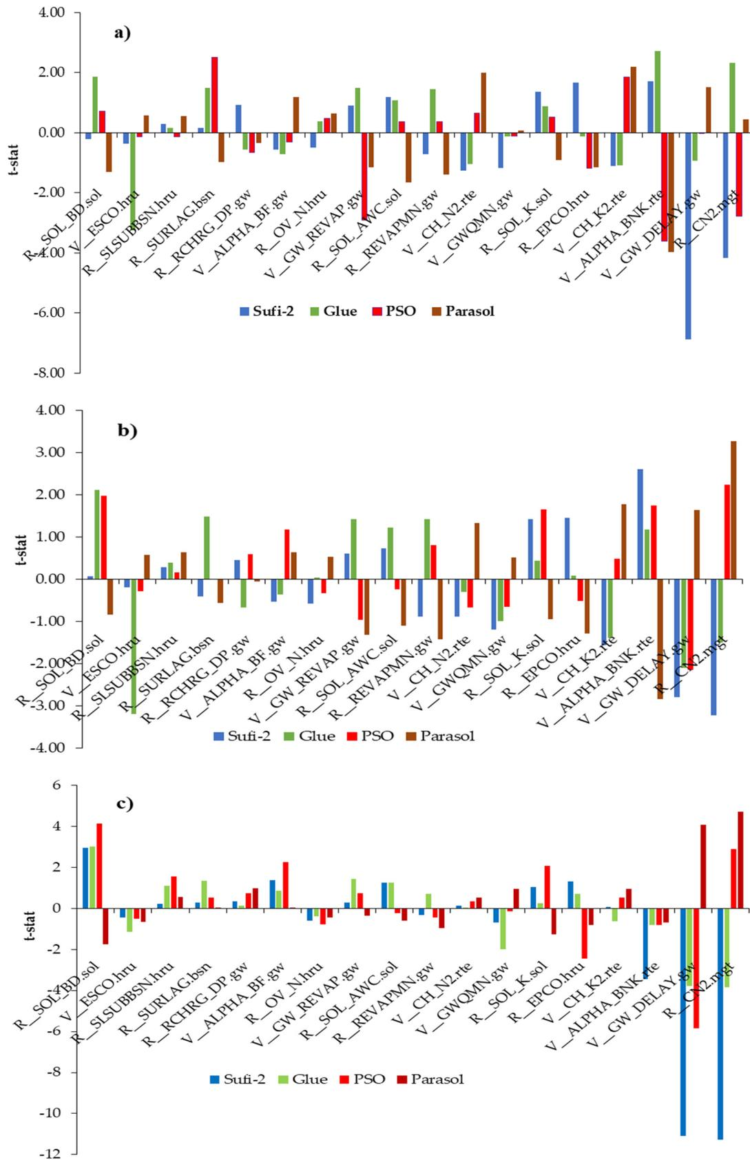
Figure 4. Sensitivity analysis of t-stat by SUFI-2, Glue, Parasol and PSO for selected sub-watersheds (a) 1, (b) 10 and (c) 23.
