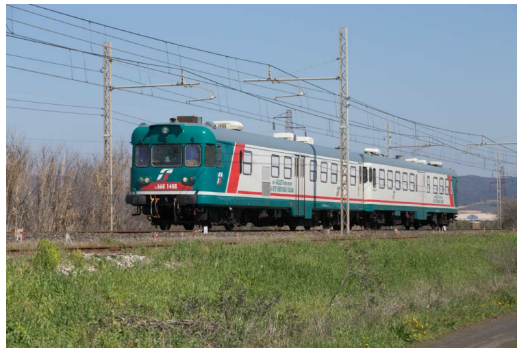
Figure 9. Ultrasonic testing vehicle “us1-Galileo” (courtesy of © Benedetto Sabatini).
