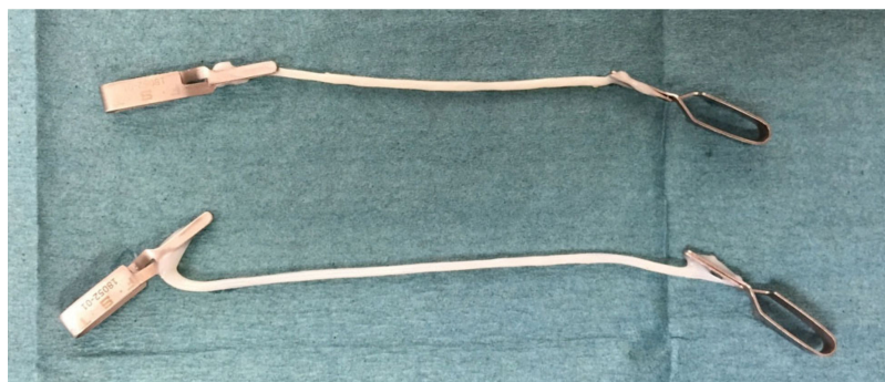
Figure 4. Tendon like constructs after 21 days of mechanical stressing using the bioreactor. The top one contains spider silk (experimental group A), the bottom one is manufactured without spider silk (experimental group B). The constructs showed phenotypes comparable to tendon tissue with no difference between experimental groups A and B.
