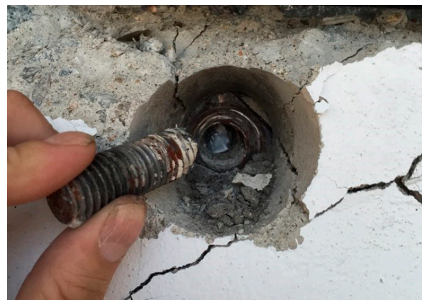
(b) Shear failure of screw rod at truss connection
