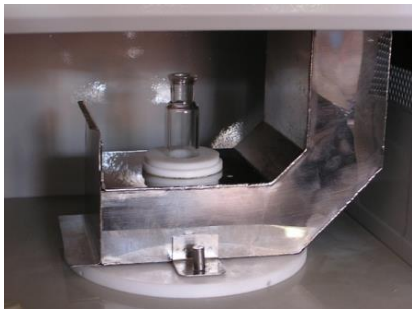
Figure 1. Glass vessel placed in the waveguide which was in the chamber of the device.
