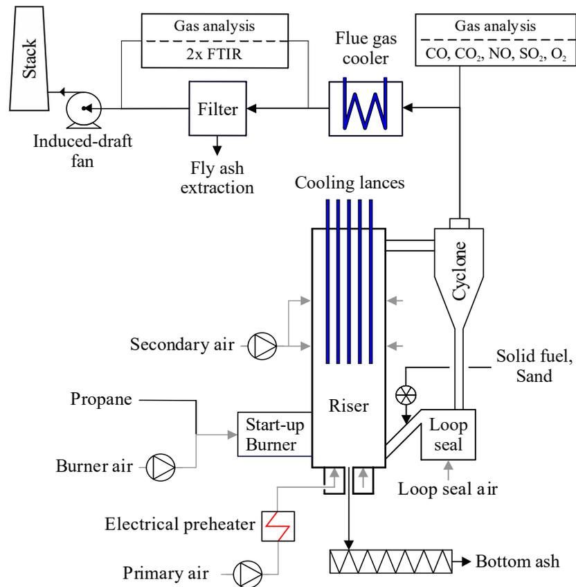
Figure 2. Simplified flow diagram of the 1 MW<sub>th</sub> pilot plant at the Technical University of Darmstadt.
