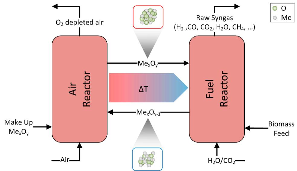
Figure 1. Schematic of the chemical looping gasification process.
