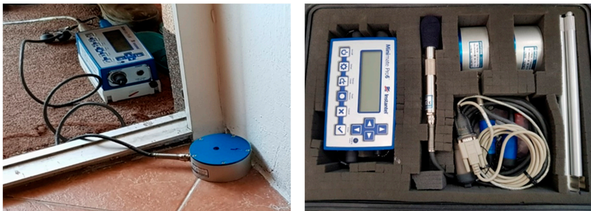
Figure 4. Placement of the vibrographs Minimate Pro 6-Position S1 (source: author).
