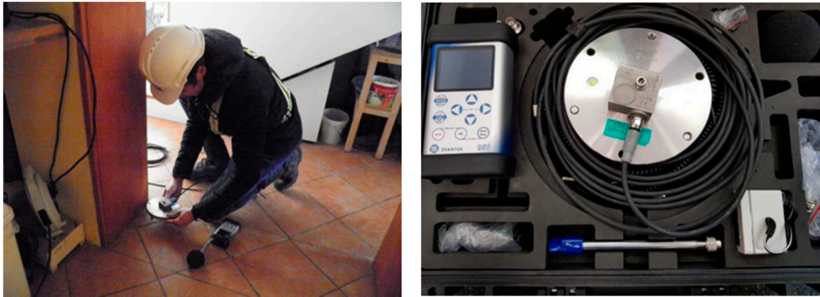
Figure 5. Placement of the vibrograph Svantek 958 A-Position S2 (source: author).
