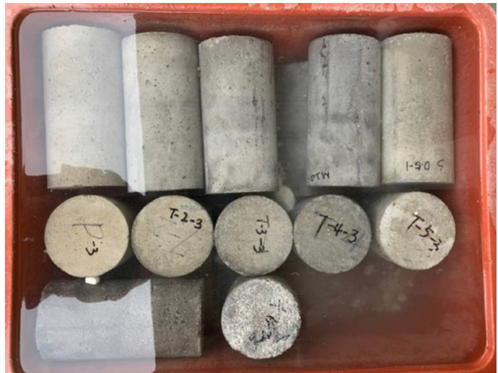
Figure 2. Immersion in sulfuric acid solution.
