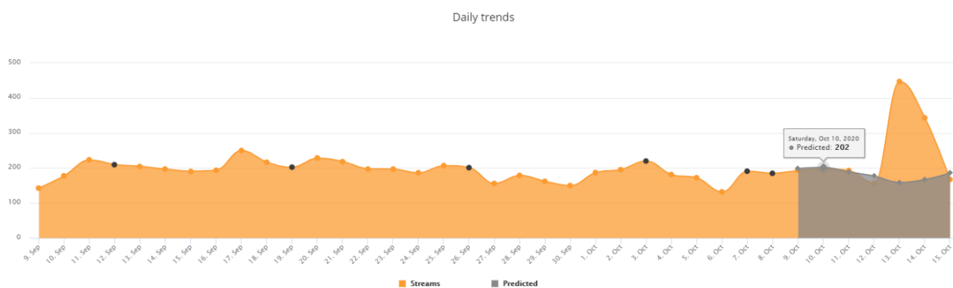
Figure 5. The presentation of outliers and explanations in DMGs monitoring system: Expected versus observed streaming count (Level 1 Explanation) are presented for each outlier and when the users hover the individual predictions the explanation of the predicted value is highlighted (Level 2 Explanation).
