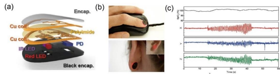
Figure 5. (a) Illustration of the various constituent layers of the NFC-enabled pulse oximeter device. (b) Photograph image of measurement setup to evaluate SpO 2 level from the fingernail (up). It is possible in application of a device with a computer mouse functioning as a wireless interface. Photograph image of measurement setup to evaluate SpO 2 level from the earlobe (down). (c) Calculated SpO 2 during rest and movement on the device. The device quantified the accelerometer's signal according to the movement in the X(red), Y(blue), and Z(green) axes. Adapted with permission from [31], Wiley, 2016.
