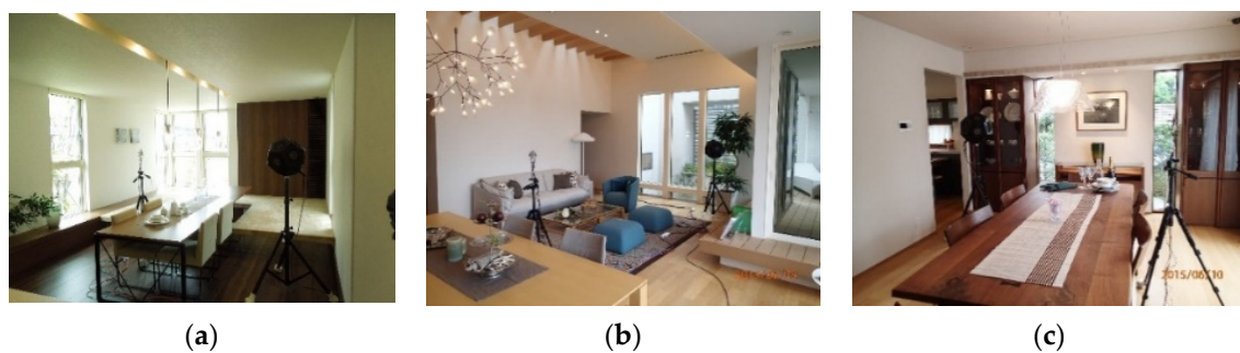
Figure 9. Measurement of impulse response in the three LD rooms: houses (a) A, (b) B, and (c) C.
