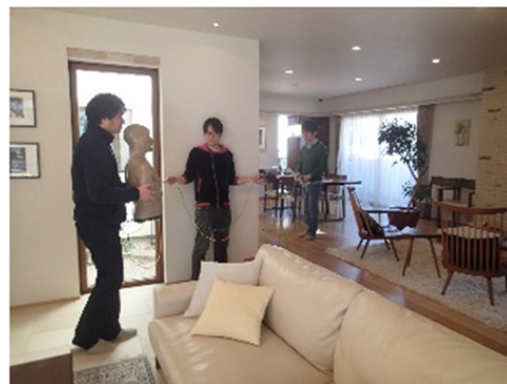
Figure 13. Binaural recording in the LD room. The experimenter holds the dummy head and walks around the room generating a footstep sound.
