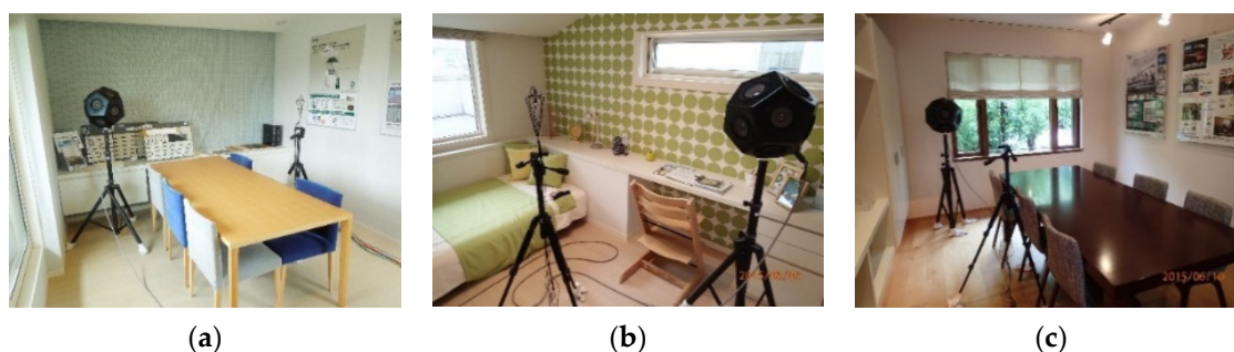
Figure 10. Measurement of impulse responses in the three child rooms: houses (a) A, (b) B, and (c) C.
