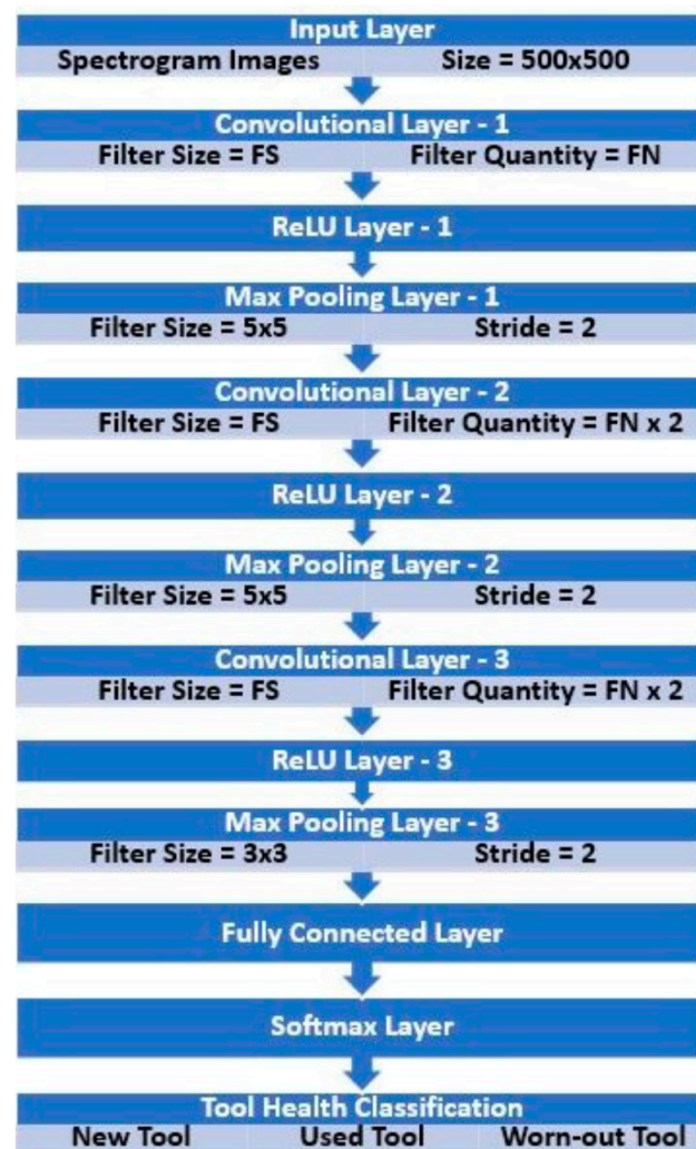
Figure 28. CNN architecture with layers sequence where FS = convolutional filter size, FN = number of convolutional filters.
