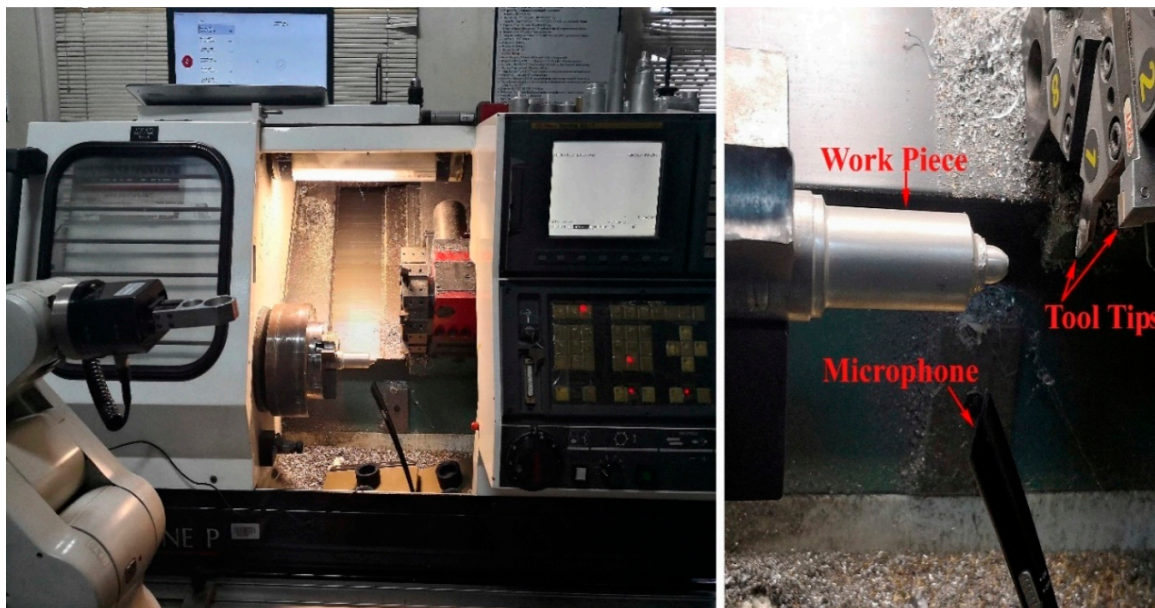
Figure 7. (Left) View of the whole experimental setup for computer numeric control (CNC) turning operation and data acquisition. (Right) Zoomed view of the setup illustrating the details of orientations.
