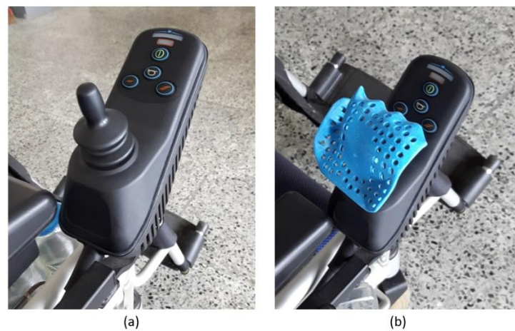
Figure 5. (a) Conventional steering controller (CSC); (b) Mounted 3D-printed steering controller (3DSC) (blue part).
