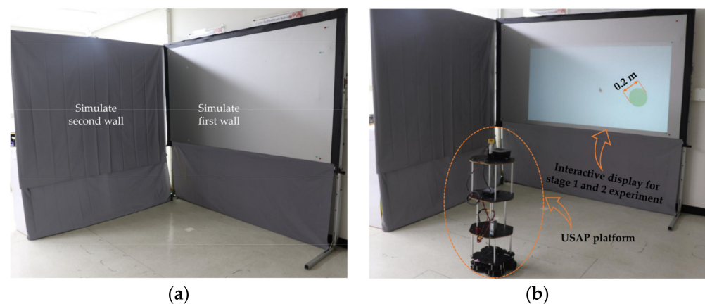
Figure 8. Experimental setup: (a) Two simulated walls; (b) the USAP platform projected onto the first simulated wall.
