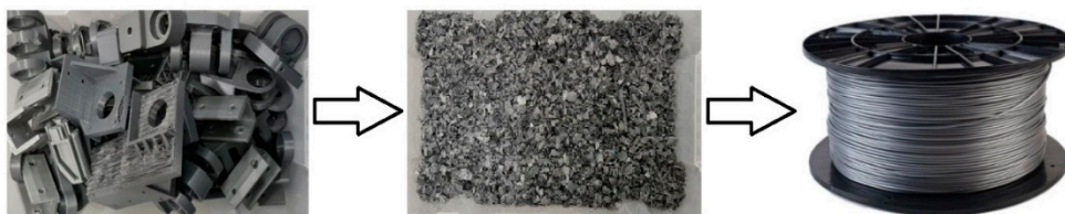
Figure 19. Demonstration of the cycle of recycling plastic models from the design of the structure.
