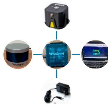
Figure 3. Processing architecture of the LiDAR (light detection and ranging).
