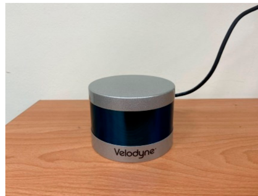
Figure 2. Velodyne LiDAR PUCK VLP-16.
