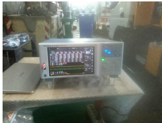
Figure 8. The Yokogawa WT 5000 instrument during the electric measurements.
