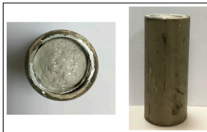
Figure 5. Samples after the foaming process and removal from the oven, ready to be extracted from the molds.
