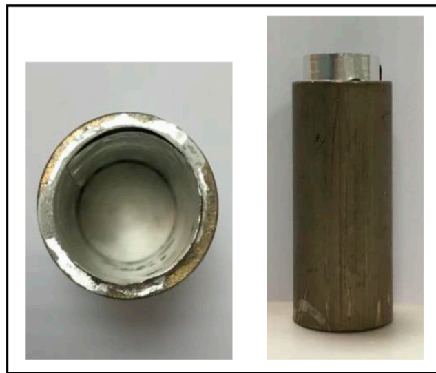
Figure 4. Prepared tablet inserted in a thick aluminum sheet, and a mold on a stainless steel base ready to be foamed.
