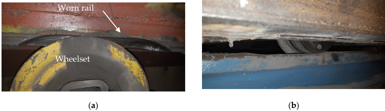
Figure 6. Example of the wear on the wheelset: (a) abrasive wear on the running rail in contact with the wheelset, (b) material loss in the running rail.
