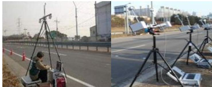
Figure 1. Vehicle velocity measurement with existing equipment.
