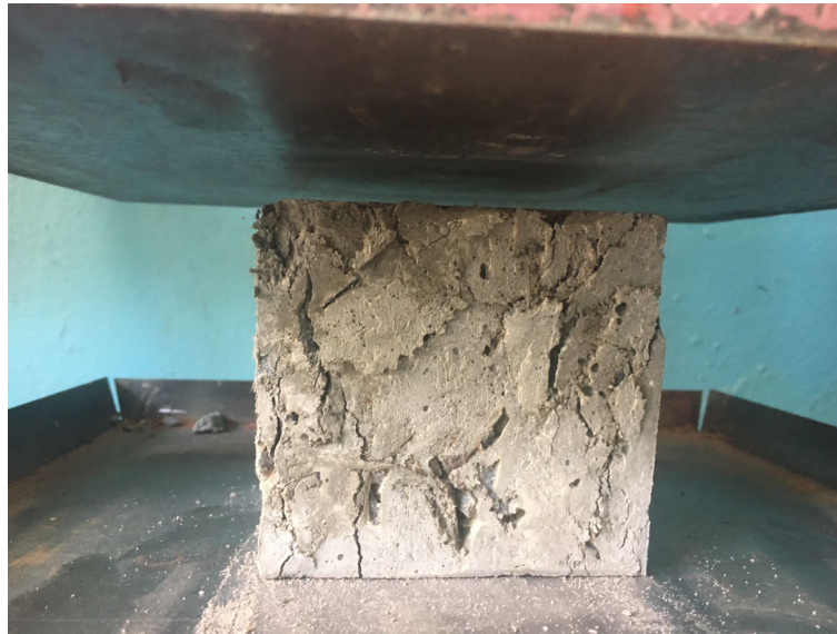
Figure 4. Sample after compression test.
