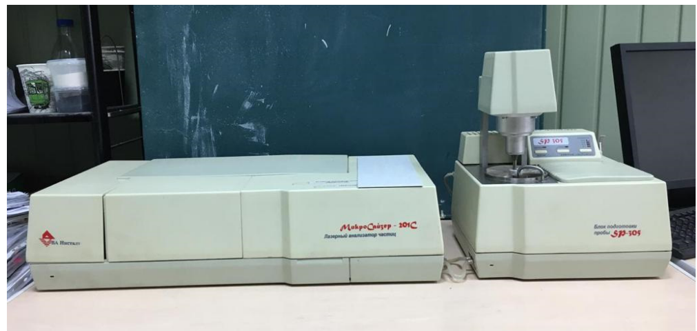
Figure 2. Laser particle analyzer Microsizer 201C.
