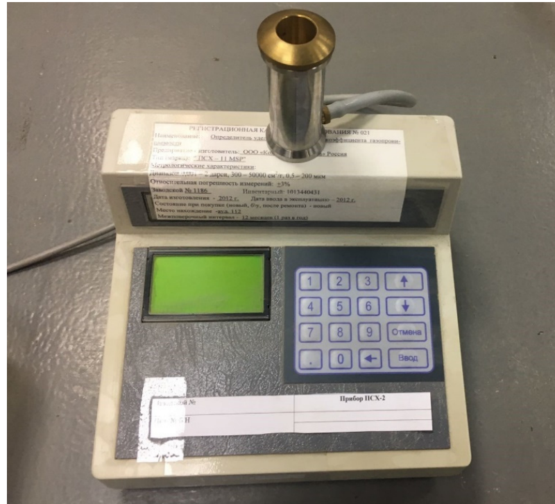
Figure 3. Device for measuring the specific surface area of particles PSKh-11 MSP.
