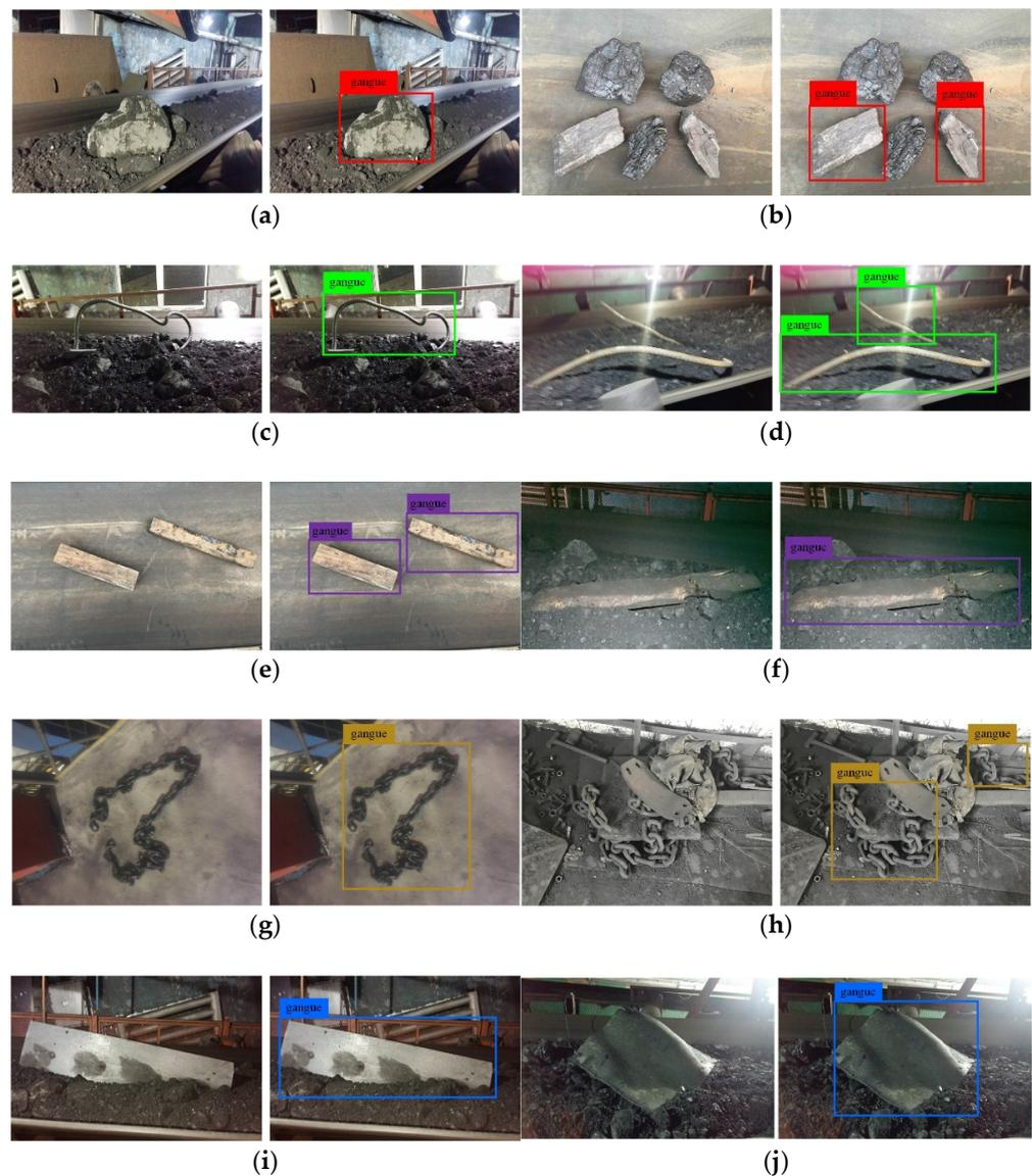
**Figure 10.** Visualization results. In the sub-figure (a–j), the left is the original picture, and the right is the visualization result of the proposed network. The sub-figures (a,b) show the detection of gangue; the sub-figures (c,d) show the detection of bolt; the sub-figures (e,f) show the detection of stick; the sub-figures (g,h) show the detection of iron chain; the sub-figures (i,j) show the detection of iron sheet.
