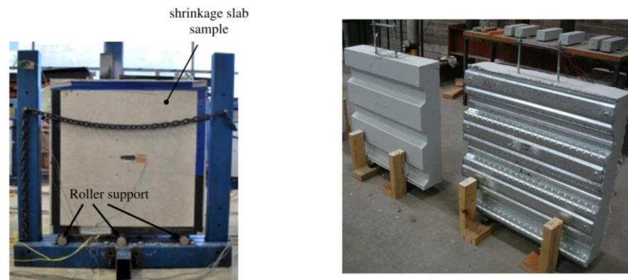
Figure 3. Typical experimental setups for measuring the characterization of the shrinkage-induced deformations [14,17].
