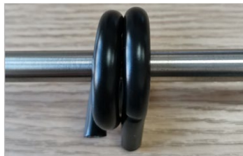
Figure 6. The shaping effect of spring cable using the wire baking method.
