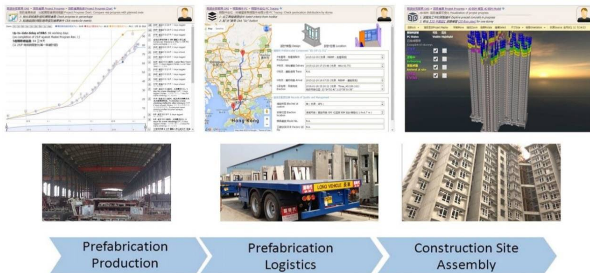
Figure 4. Visibility tools for MITBIMP. Reprinted/Adapted with permission from Reference [35]. Copyright 2017 Copyright Elsevier B.V.
