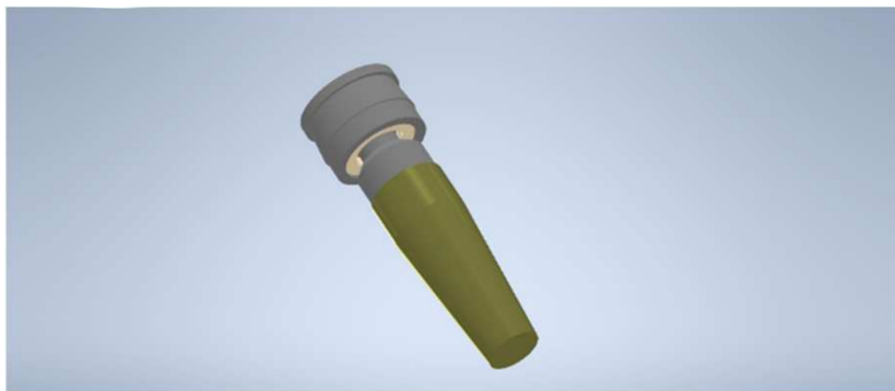
Figure 3. The 3D Model of the implant and ball attachment, with matrix housing.
