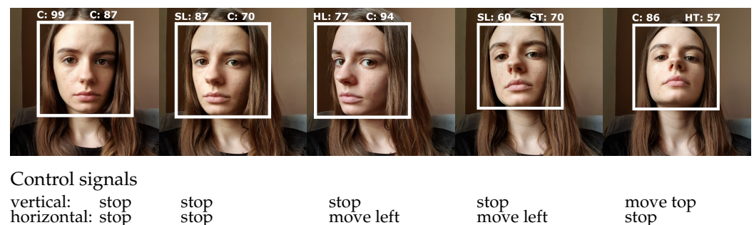
Figure 8. Video frames from the camera pointed at the operator's face. The white rectangle represents the head bounding box, whereas the values above describe the head estimation output class, together with probabilities.
