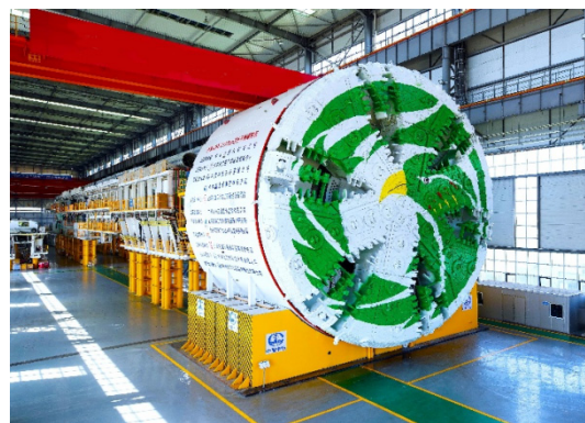
Figure 3. Slurry shield of the Chunfeng tunnel.
