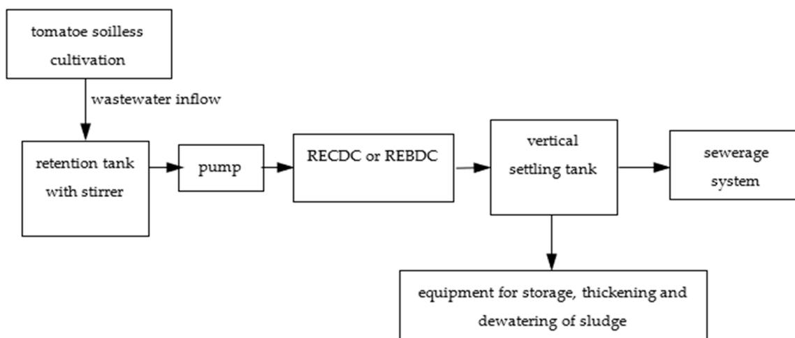
**Figure 6.** Scheme of a technological system with electrochemical or electrobiological rotating disc contactors for treating wastewater discharged to sewage systems.
