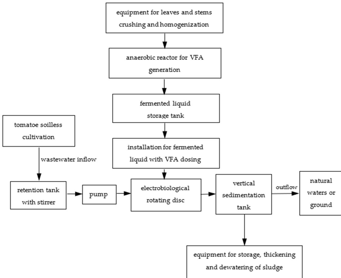
**Figure 8.** Scheme of a technological system with an electrobiological rotating disc contactor with equipment for VFA generation from leaves and stems crushing, for treating wastewater discharged into natural waters or the ground.
