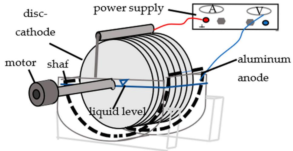
**Figure 1.** Scheme of the unit experimental model.
