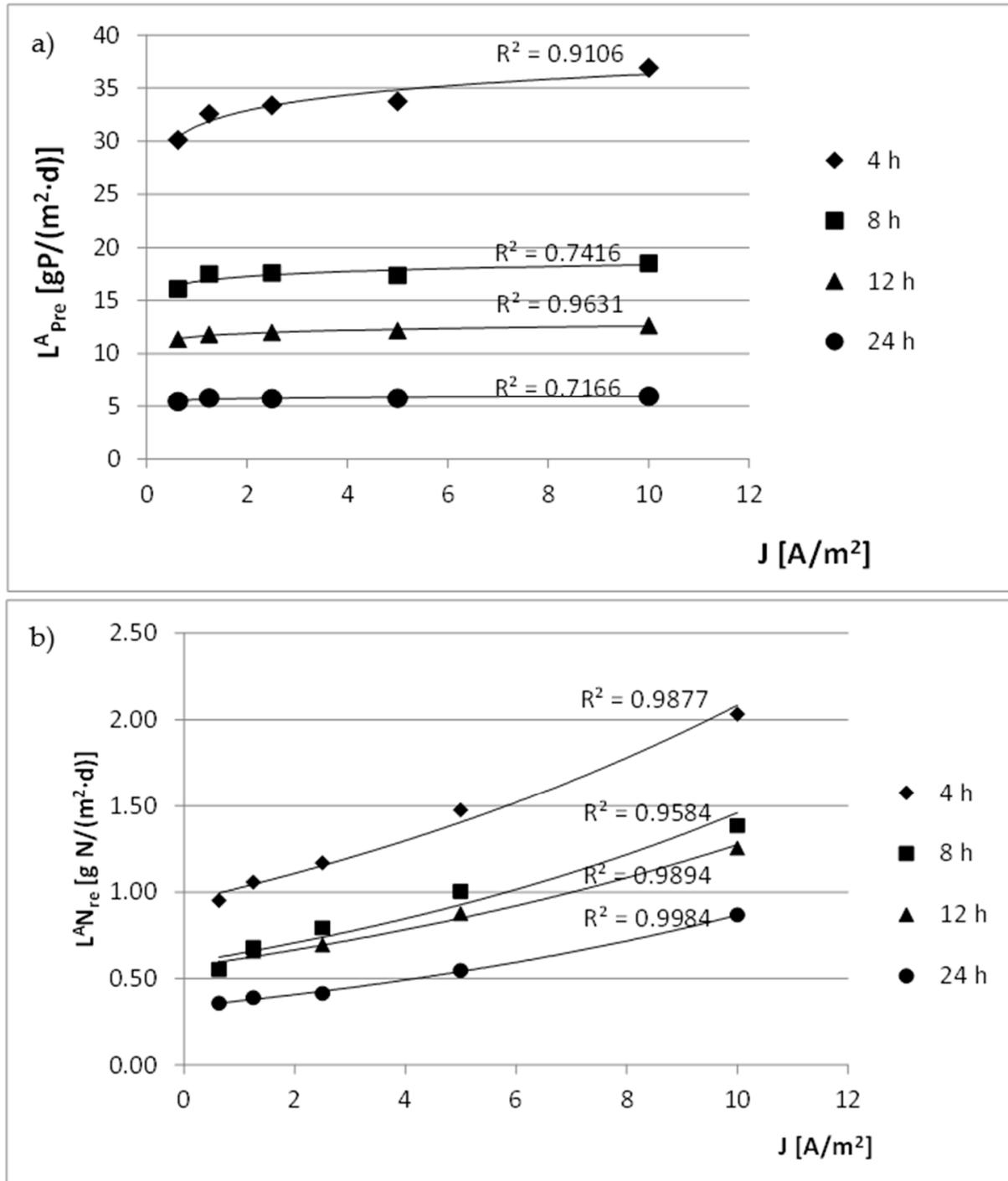
**Figure 2.** The influence of current density and HRT on the removed load ( $L^A$ ) per day in the electrochemical rotating disc contactor (RECDC): (a) Phosphorus ( $L^A_{Pre}$ ); (b) total nitrogen ( $L^{AN}_{re}$ ).
