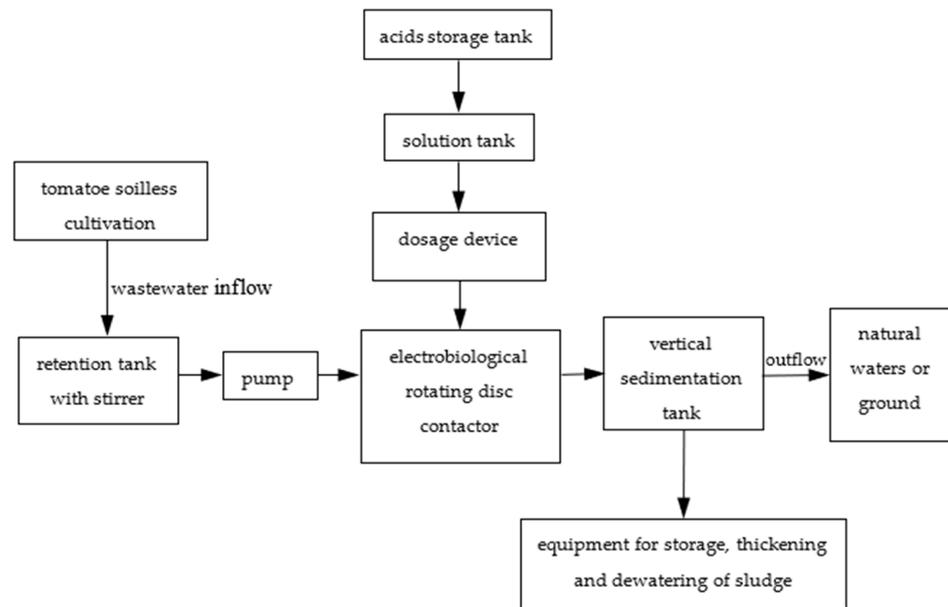
**Figure 7.** Scheme of a technological system with an electrobiological rotating disc contactor with external carbon source for treating wastewater discharged into natural waters or the ground.
