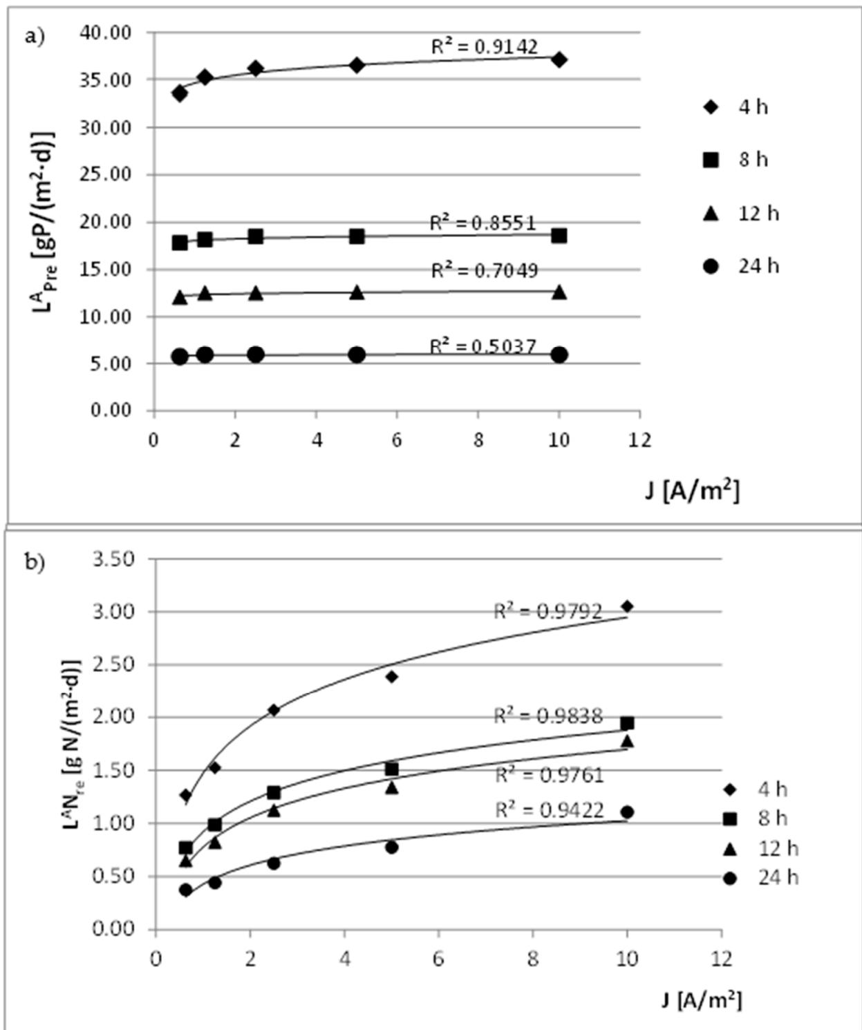
**Figure 3.** The influence of current density and HRT on the removed load per day ( $L^A$ ) in the electrobiological rotating disc contactor (REBDC): (a) Phosphorus ( $L^A_{Pre}$ ); (b) total nitrogen ( $L^A_{Nre}$ ).
