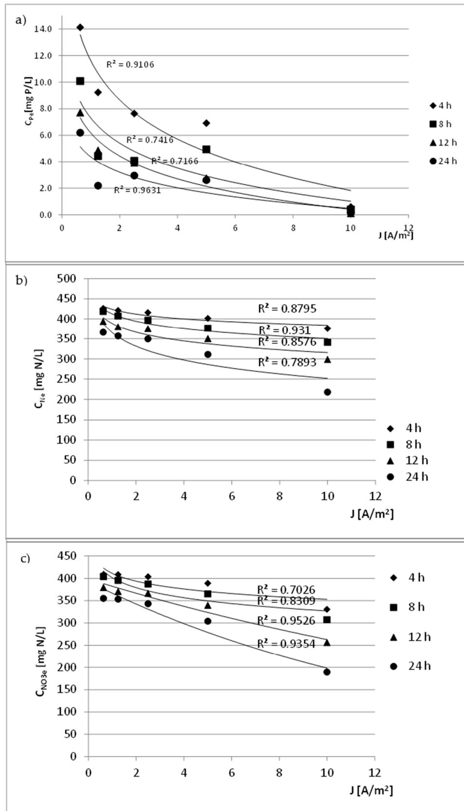
**Figure 4.** The influence of current density and HRT on the concentration of pollutants in the treated wastewater in the electrochemical rotating disc contactor (RECDC): (a) Phosphorus ( $C_{Pe}$ ); (b) total nitrogen ( $C_{Ne}$ ); (c) nitrates ( $C_{NO3e}$ ).
