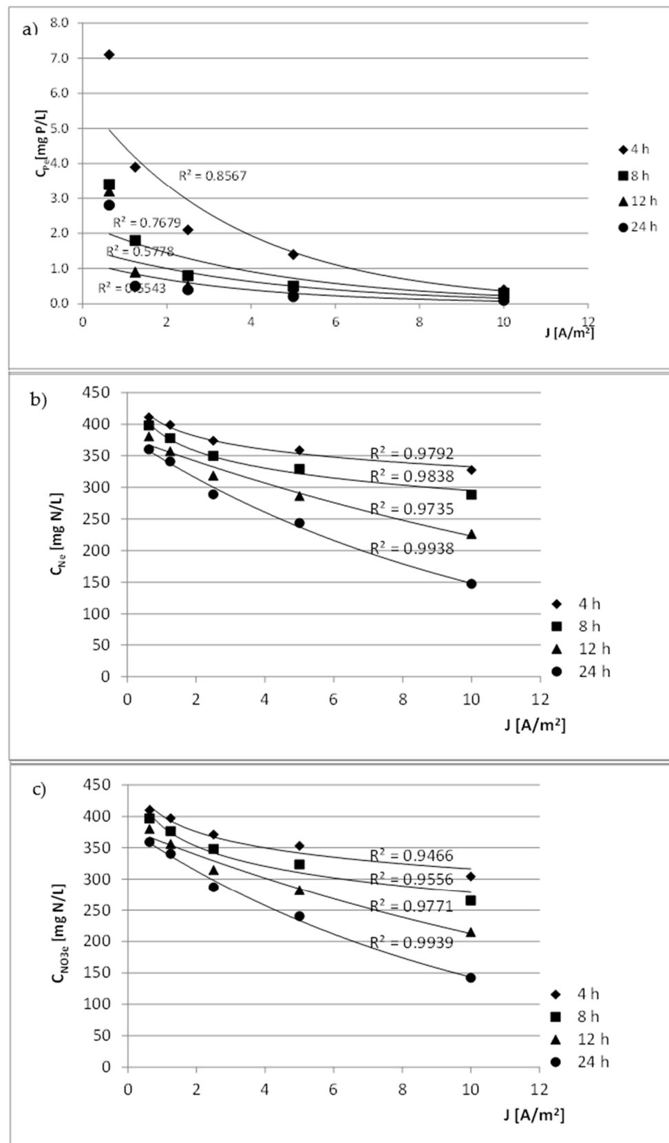
**Figure 5.** The influence of current density and HRT on the concentration of pollutants in the treated wastewater in the electrobiological rotating disc contactor (REBDC): (a) Phosphorus ( $C_{Pe}$ ); (b) total nitrogen ( $C_{Ne}$ ); (c) nitrates ( $C_{NO3e}$ ).
