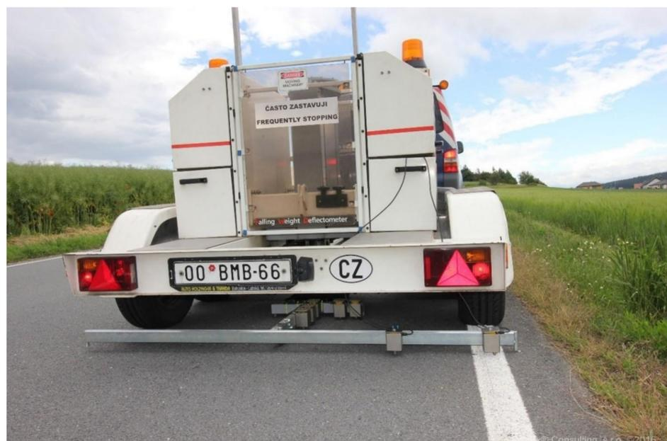
**Figure 3.** Layout of an auxiliary cross frame.
