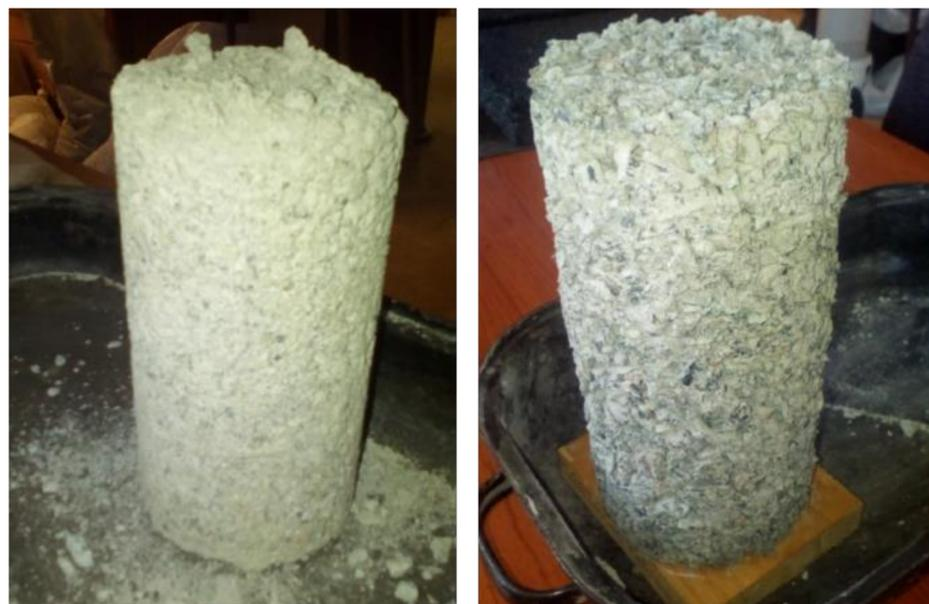
Figure 5. Specimens for CTT: GM 0/22 (left); GM 0/32 (right).
