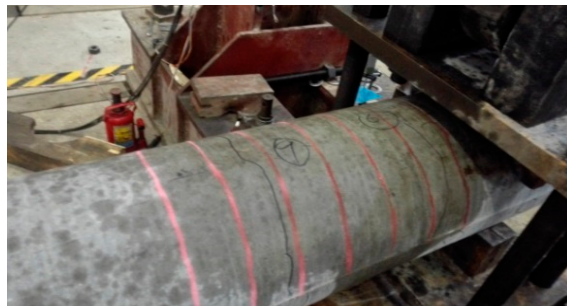
Figure 7. The crack development of PHC tube column specimen during loading.
