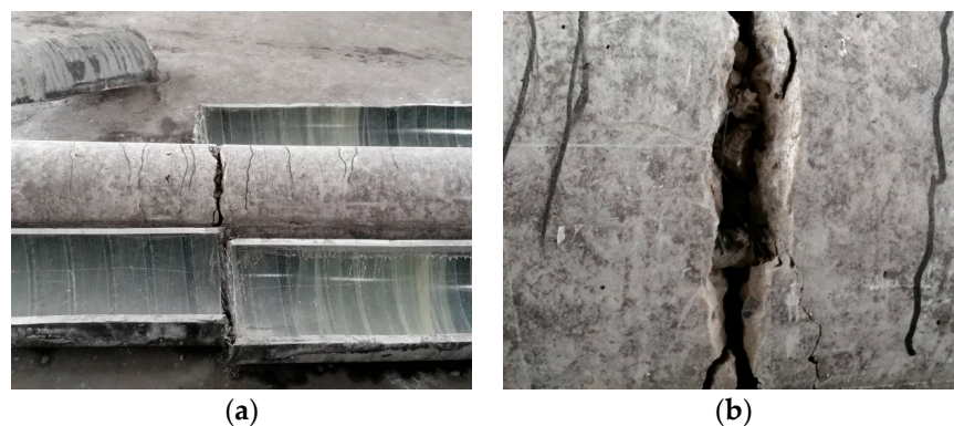
Figure 9. The crack development in the internal concrete of the BFRPC composite column specimen: (a) Overall view of cracks; (b) crack in the mid-span.
