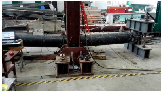
Figure 8. The test phenomenon of the BFRPC composite column specimen.
