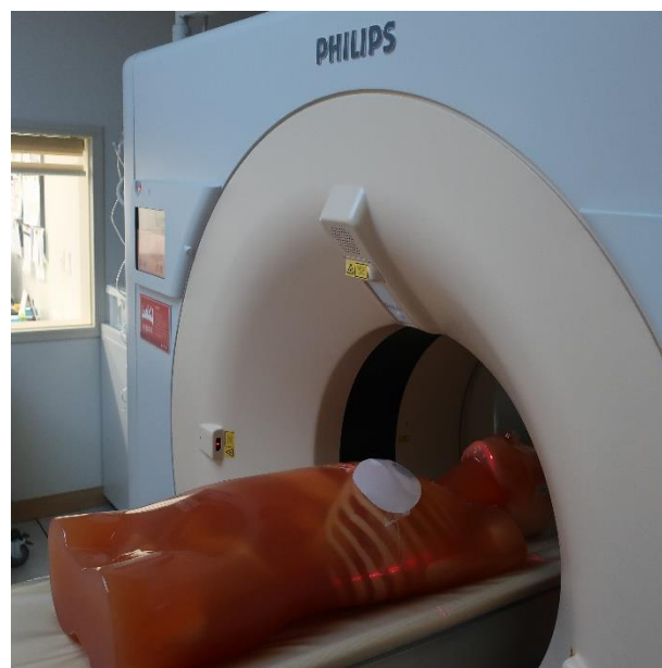
Figure 2. Computed tomography simulation. A tissue expander was attached to the left chest wall of the phantom.
