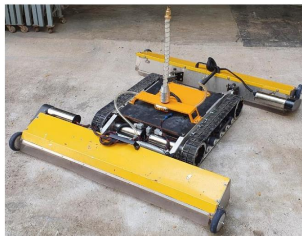
Figure 6. Prototype of PV cleaning robot.
