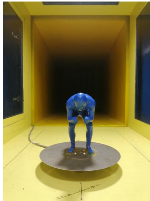
Figure 7. Scale models in the wind tunnel.
