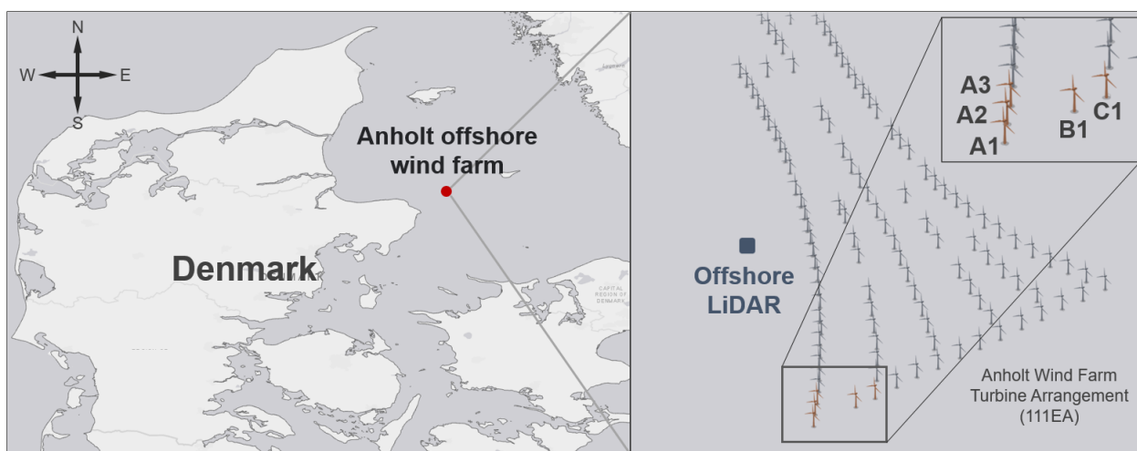
Figure 1. Left: Location of the Anholt offshore wind farm. Right: Arrangement of 111 offshore wind turbines. The offshore LiDAR is marked as dark-blue square to the west of Anholt wind farm. Only the five identified wind turbines (A1–A3, B1, and C1) marked in orange color in the enlarged figure are used for this analysis.
