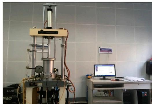
**Figure 1.** TYD-20 dynamic triaxial test apparatus.
