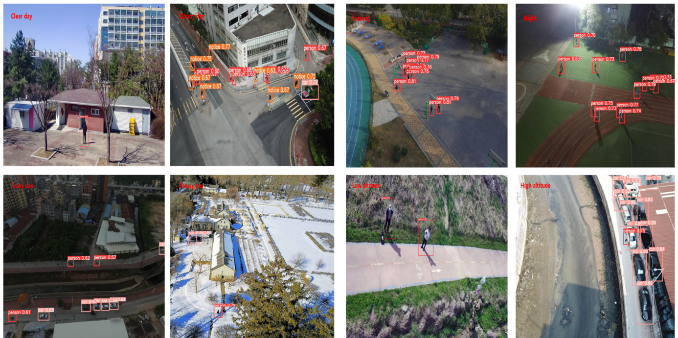
Figure 13. Detection result for the YOLOv5_Ours model (Red is person, Orange is notice, and Pink is car).
