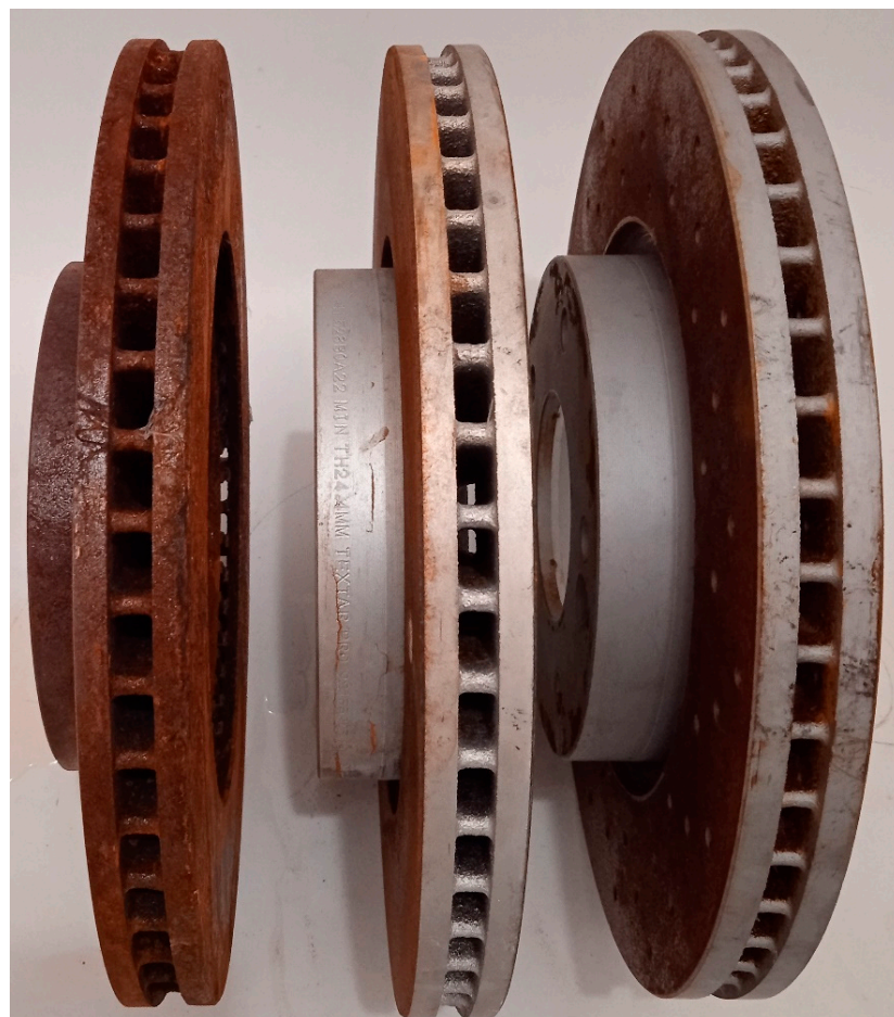
Figure 19. Corrosion on the sides of brake discs.
