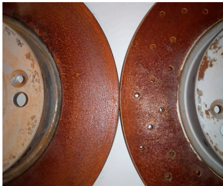
Figure 21. Corrosion on the friction area of mid-priced and high-priced brake discs.
