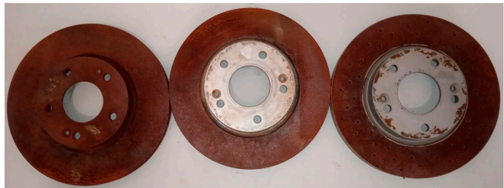
Figure 17. Corrosion on the outer side of brake discs.
