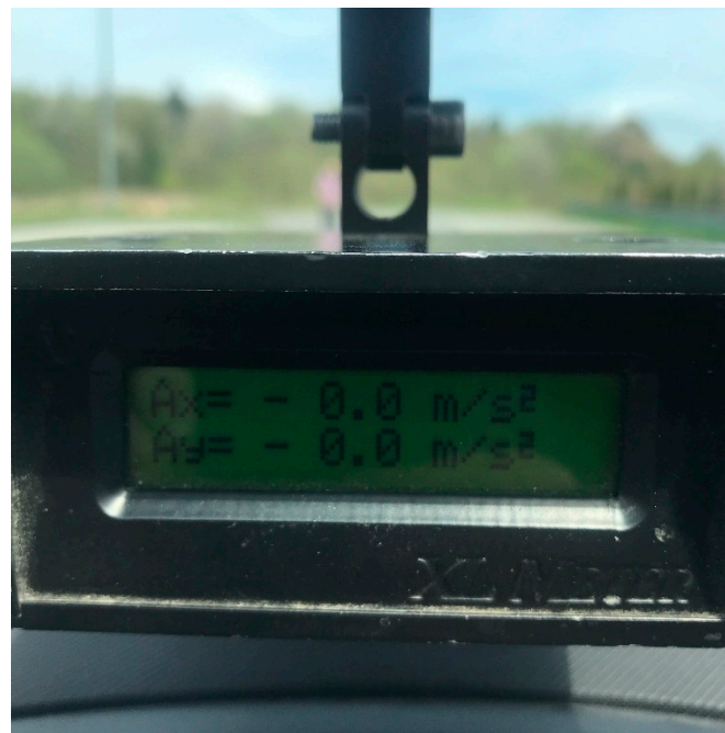
Figure 2. Decelerometer used for measuring.
