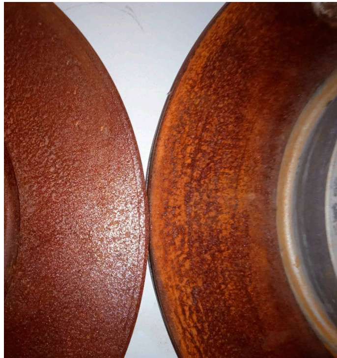
Figure 20. Corrosion on the friction area of low-priced and mid-priced brake discs.
