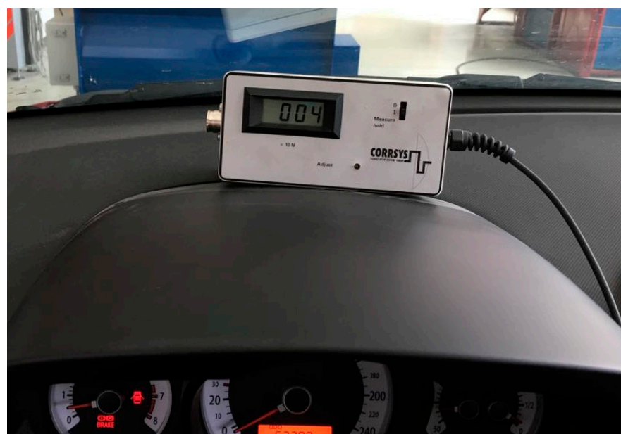
Figure 4. Pedometer used for measuring the effort to control the steering affecting the brake pedal.
