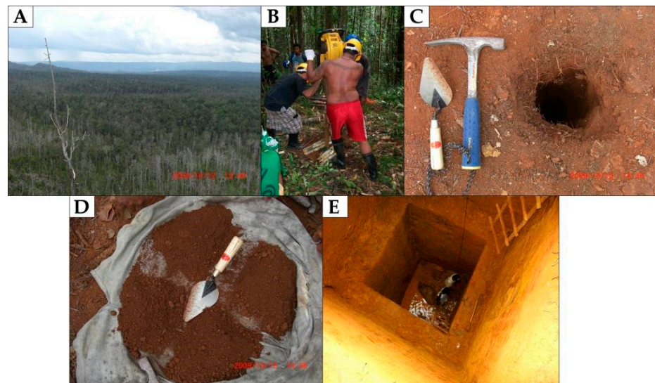
Figure 3. (A) The forested area of Weda Bay where prospecting works were conducted, (B) sampling using a hand-held impact sampler, (C) borehole, (D) coning and quartering of laterite samples, and (E) trench excavated for sampling and macroscopic description of ore structure (Photo G. Konopka).
