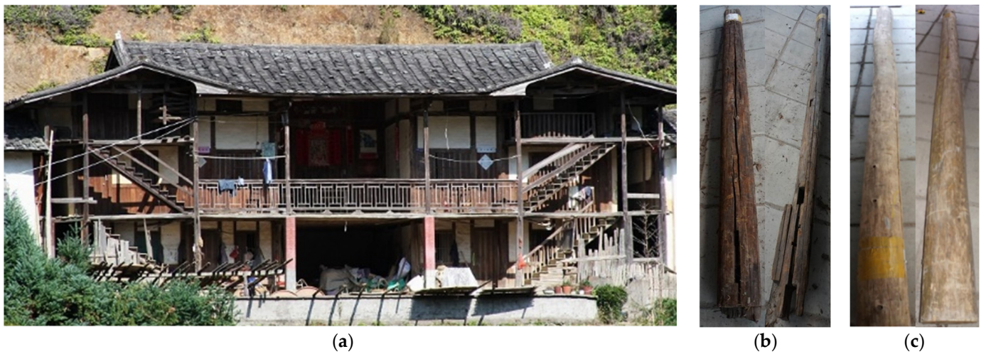
Figure 3. Log samples of aged CL and new CL: (a) hundred-year-old building, (b) aged CL samples, and (c) new CL samples.
