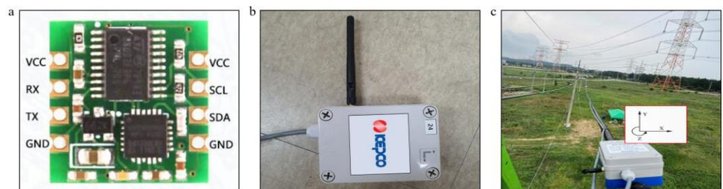
**Figure 2.** (a) WT61 module. (b) Utilized acceleration sensor in KEPCO. (c) Example of installed acceleration sensor in KEPCO.
