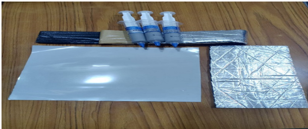
Figure 7. Thermal paste, arrays and insulators used in the panel.
