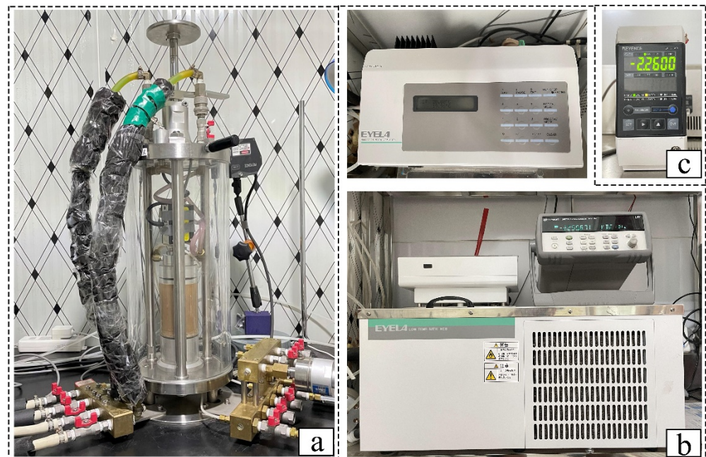
Figure 3. The main instrument used in the experiment: (a) Precision frost heave triaxial instrument; (b) Constant temperature water tank; (c) Data collector.
