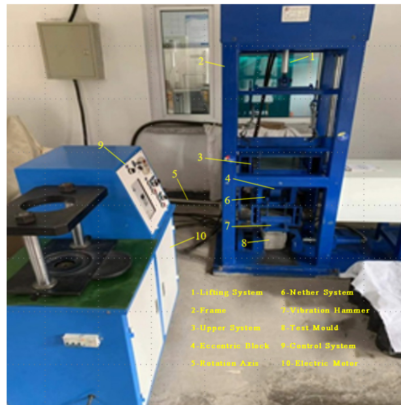
Figure 1. Schematic diagram of the structure of the vibration meter used in this study.
